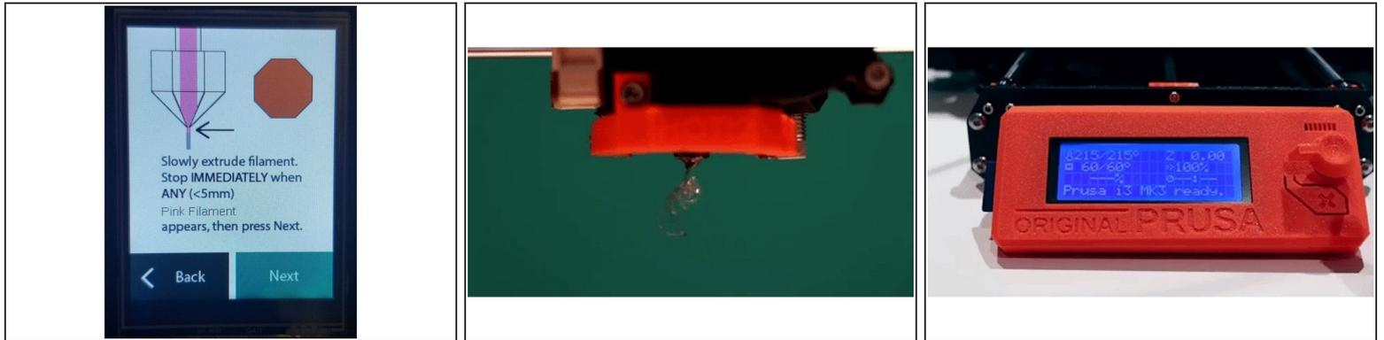
**⚠** Jog the filament through your extruder until the new colour appears. The clear filament you loaded previously will eventually change to the colour from Input 1. Stop extruding as soon as you see any hint of the filament from Input 1 appear, and confirm loading is complete on Palette's screen by selecting **Next**.
