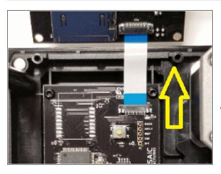
If you're still not able to read the files properly, we can check the connection of the SD card reader to the electronics tray as a last resort. Please follow these steps to remove Palette's bottom casing and access the electronics board. Unscrew the top electronics board to access the blue ribbon that you see in the picture below.
