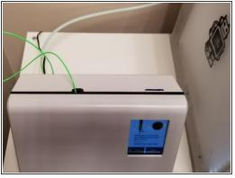
Follow the onscreen instructions to clear the outgoing tube which you would have already completed in step 3. Load filament into the inputs, making sure not to clear filament for any inputs as clear filament is used later in the calibration process. Allow Palette 2 to output filament with the outgoing tube disconnected.
