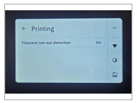
Go to Settings > Printing to turn on filament run-out detection.
