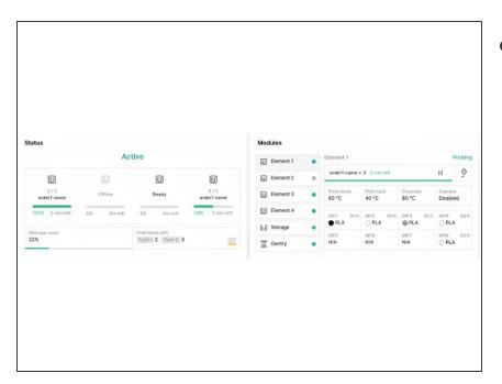
After sending to printer, navigate to the 'Devices' tab to monitor the print from the device control screen
