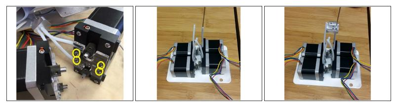
• Pull out and isolate the drive sets as you will want to work with them one at a time. Take off the acrylic drive plate on one set by removing the highlighted fasteners for each pair.
